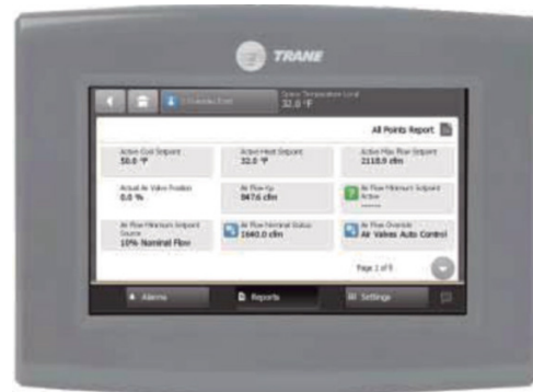
Figure 6 - TD7 operator interface
